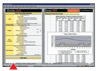
Within minutes of installing ExceLINX-1A on a PC, users can acquire data directly from the Model 2700/2750 instruments, then employ Excel's graphics, charting, and analysis capabilities to turn that data into useful information.
